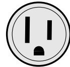
Two-Pole, 3-wire Grounding Receptacle 15 Amps. 125V.
