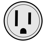
Two-Pole, 3-wire Grounding Receptacle 15 Amps. 125V.
