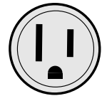
Two-Pole, 3-wire Grounding Receptacle 15 Amps. 125V.
