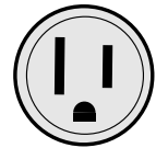
Two-Pole, 3-wire Grounding Receptacle 15 Amps. 125V.
